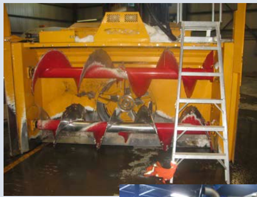
Photo 1: Auger of a snowblower.
