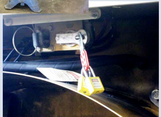
Photo 4: Key-operated battery cutoff that can be locked out with a latch.
