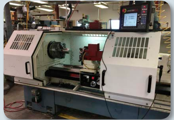
Photo 2: CNC milling machine with sliding access doors that are interlocked to the machine's power supply.
