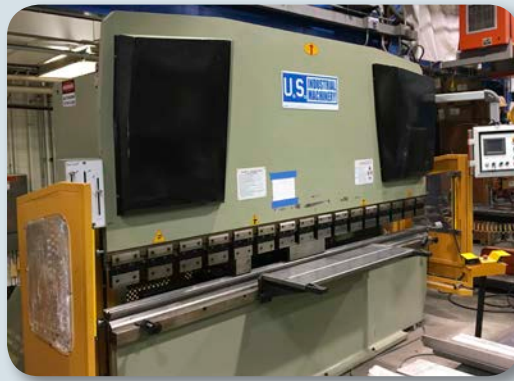
Photo 1: Hydraulic press brake equipped with presence-sensing device and two-hand actuators on the operator's control bar.
