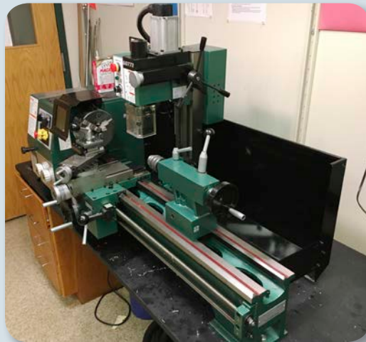
Photo 3: Satellite machine shop that includes a tabletop mill-lathe combination machine with chuck guards that are interlocked to the power supply.
